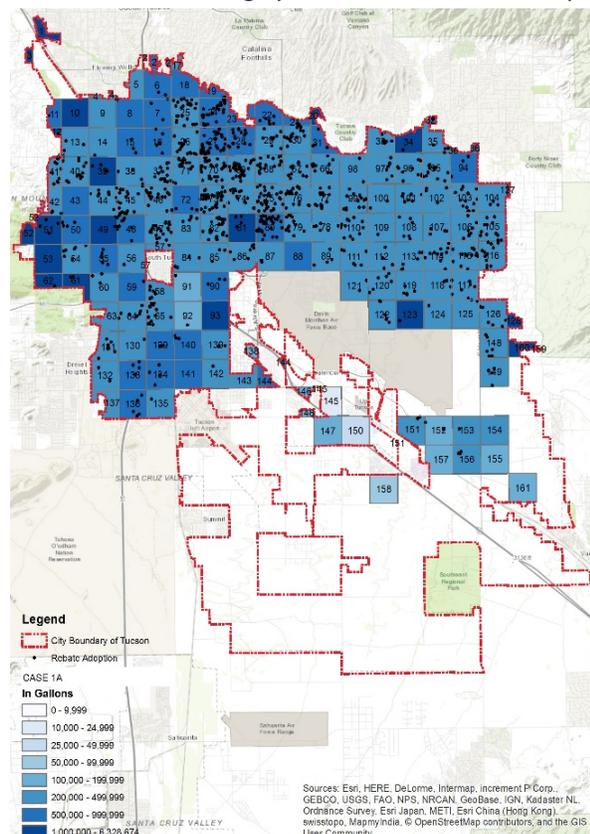
Figure 23 (left) Optimized Storage Volume for Water Independence Case 1A
