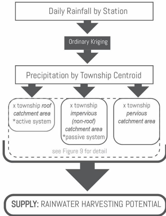
Figure 7 Rainwater Harvesting Potential with Precipitation
