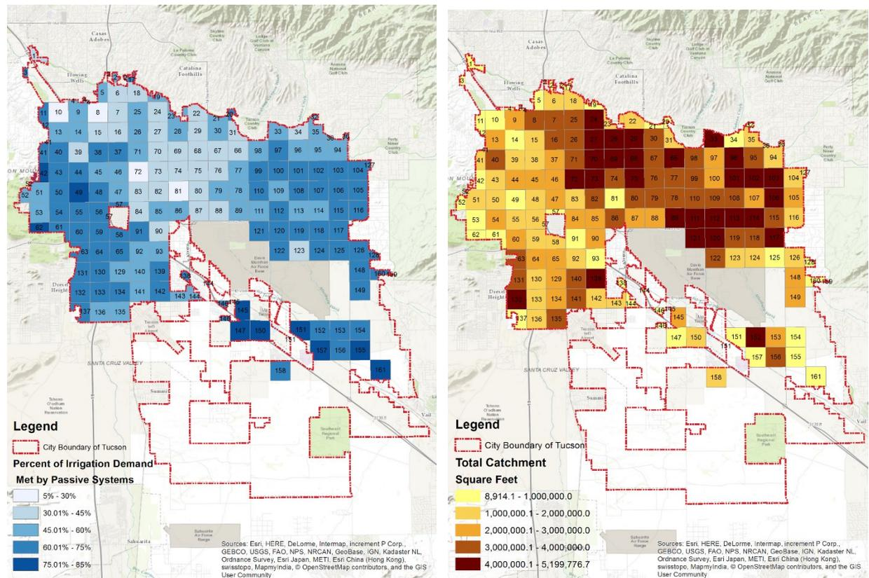
Figure 20 (left) Percent Irrigation Demand Met by Passive Rainwater Harvesting (2007-16)
