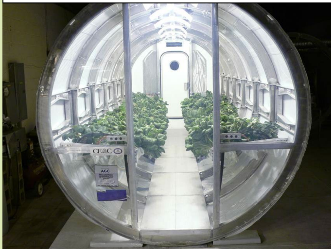
Figure 1. Prototype BLSS Lunar Greenhouse (LGH) with Cable Culture currently in operation at UJA-CFAC 8
